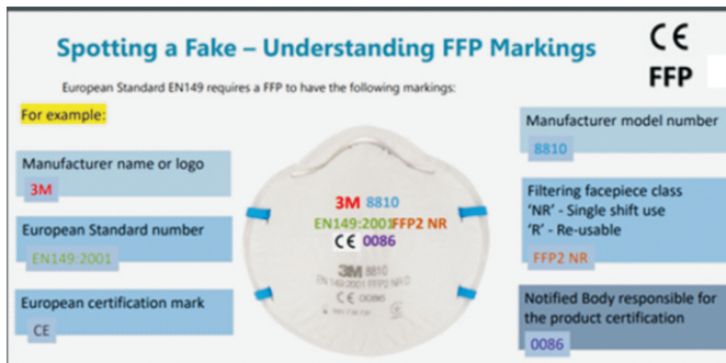
Fig 4: Markings on facepiece of FFP masks
