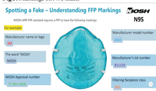
Fig 3: Markings on N95 mask
